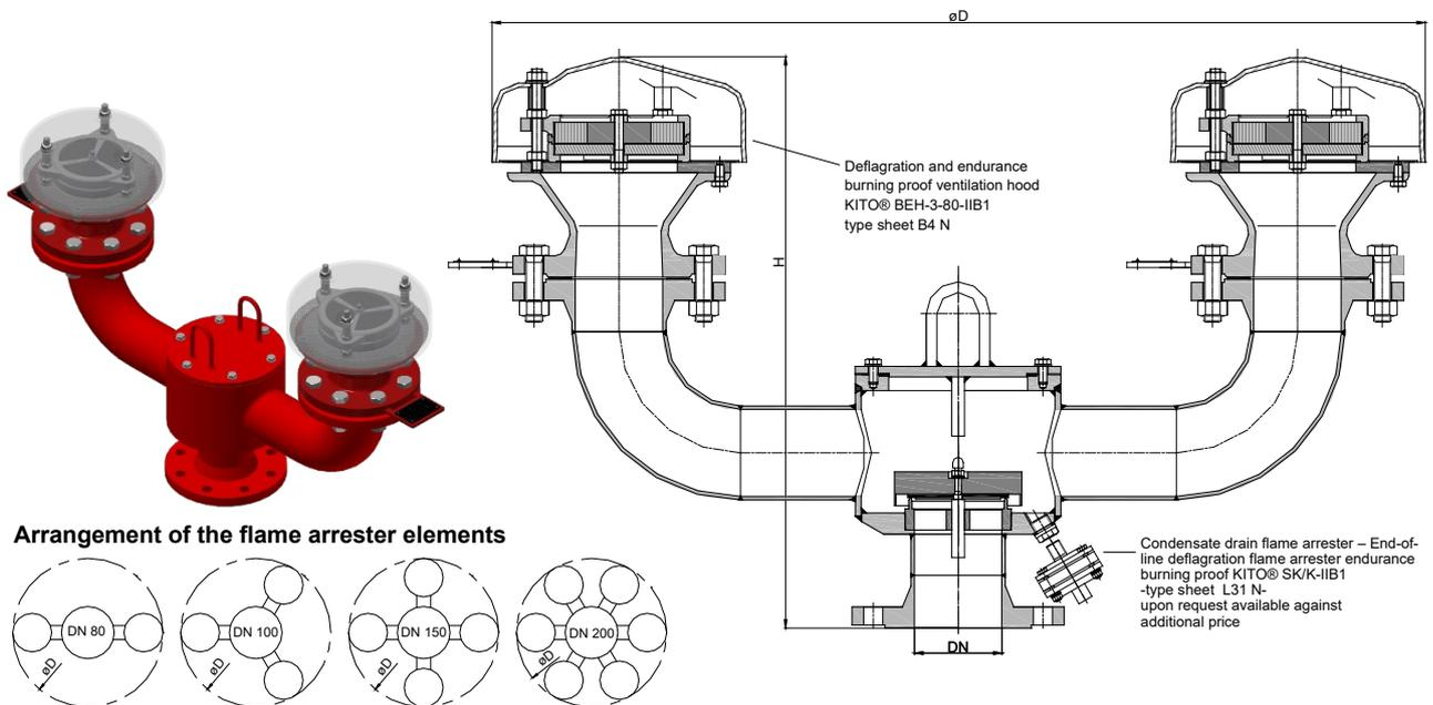
Arrangement of the flame arrester elements
